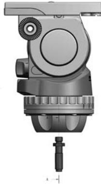
If you want to fit the FSB 6 onto on a flat base, remove the threaded pin.
